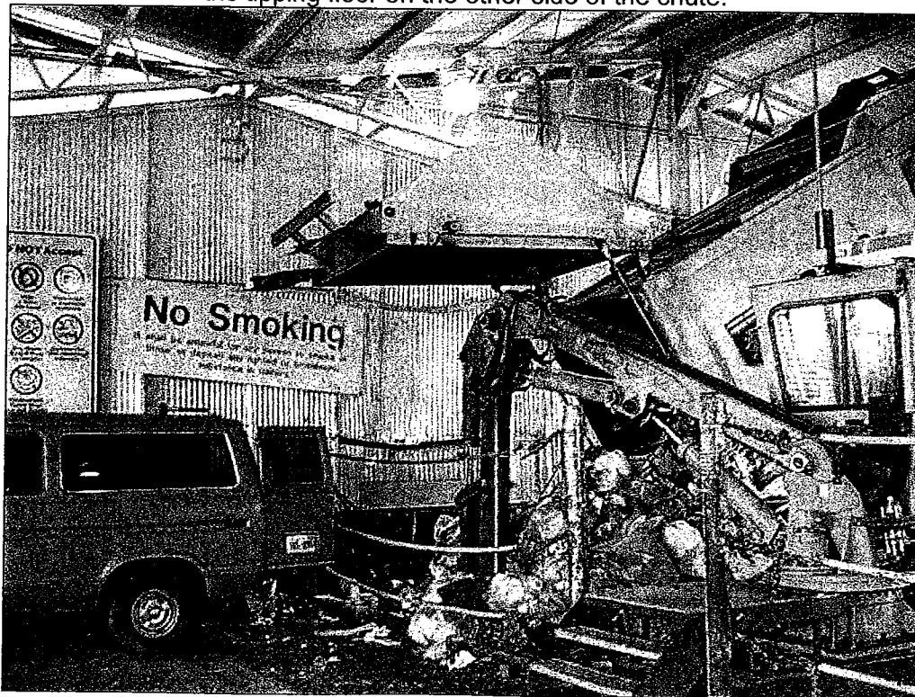
The back door of a commercial vehicle opens over a self-haul vehicle while dumping garbage into the same chute.
